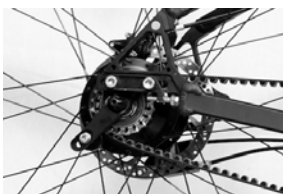
Illustration 3: Side view of the installed Snubber
