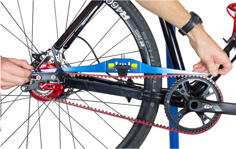
Illustration 2: Checking the belt tension in the load strand
