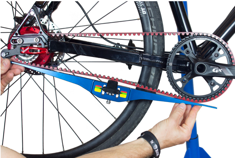
Illustration 3: Checking the belt tension in the return strand
