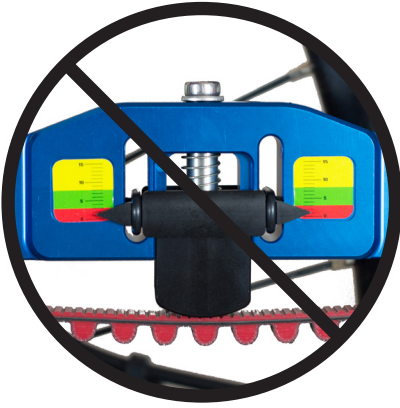
Illustration 1: Incorrect belt tension
