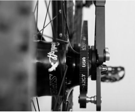
Illustration 3: Correct alignment of the belt
