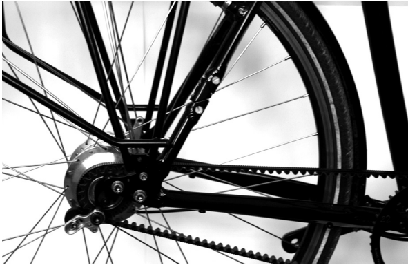
Illustration 3: Example for frame construction: separation of the seat stay
