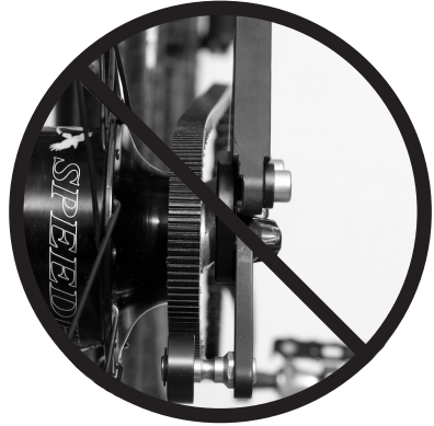
Illustration 4: Incorrect alignment of the belt
