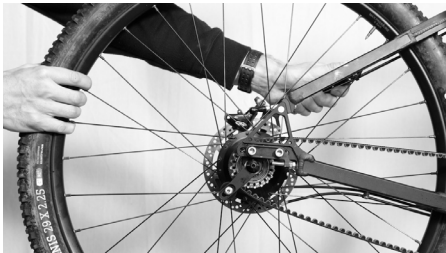
Illustration 3: Correct alignment of the belt
