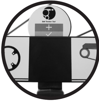
Illustration 3: Optimal belt tension
