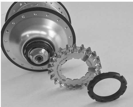
Illustration 1: Rohloff SPEEDHUB 500/14 with Splined Carrier and Lock-Ring
